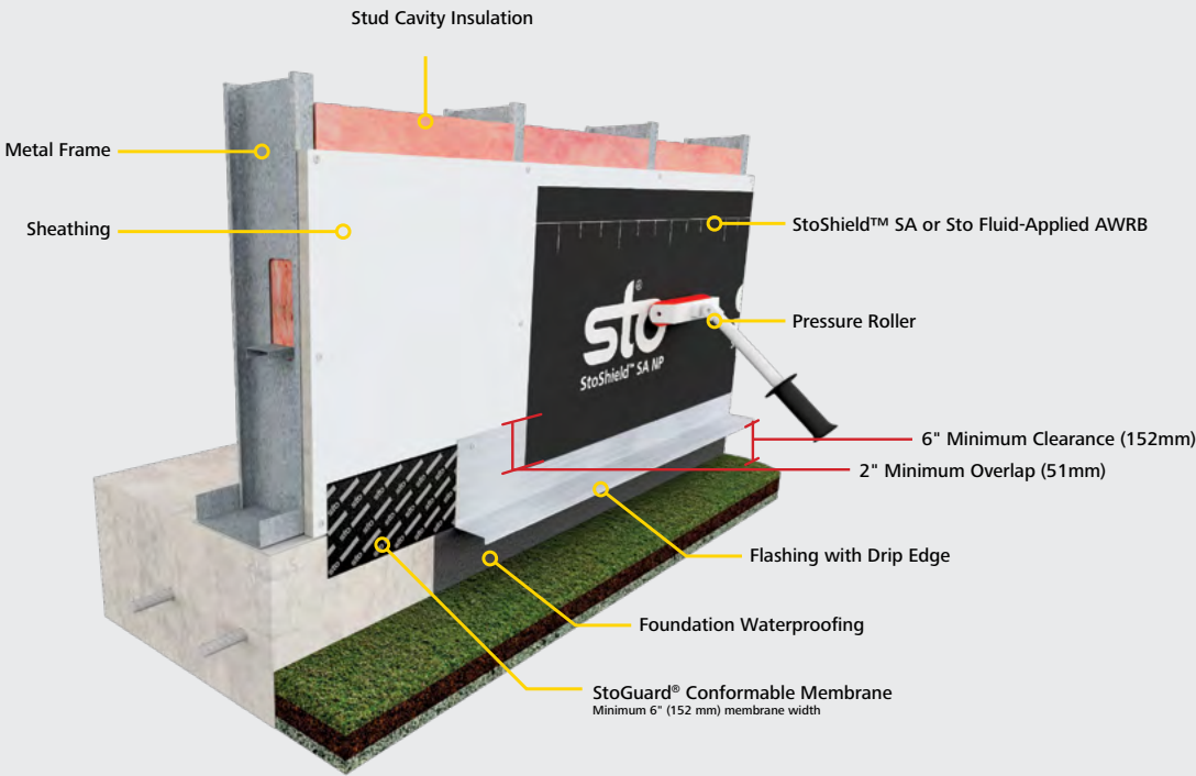
StoShield™ SA AWRB with StoGuard® Termination at Grade Detail
